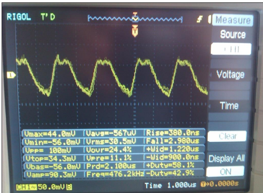
Figure 5. Intensity modulation of a square wave
